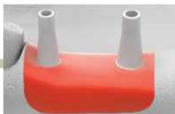
Seat Burn-Out Cylinder securely into the Lab Analog on the master cast.
