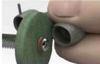
Trim extended margin with rubber wheel
