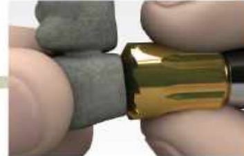
Reamer is used to eliminate lip caused by 'snap-on' mechanism.
